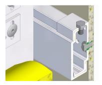
Because of the nature of the invisible mechanical fixing, it is required to install the panels from bottom to top, it is not practical for an installer to adjust and fixate the panel hangers unless there is sufficient free space above the panel. The panels are supported individually and they do not rest on each other (8mm joint around each panel), so the edges are not damaged.
