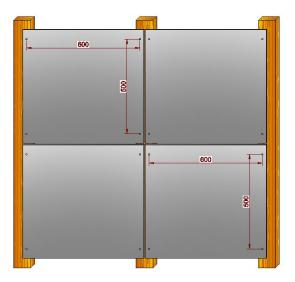
• 3x3 Configuration or more: If the façade panel is installed with 9 or more mountings, this is possible with spacings of 600 x 600 mm. Smaller spacings are also possible, but then the number of profiles of the supporting structure increases and the dimensions of the façade panels become smaller.
