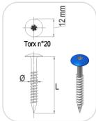
Façade panel screw, timber screw with painted mushroom head Ø 12 mm, Torx impact no. 20.
