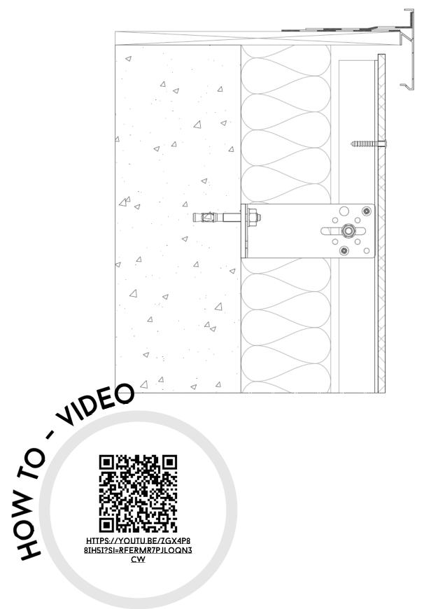
Always provide an expansion joint of at least 8mm if the façade panels connect to another element such as a brick wall, a garden house with wooden cladding...
