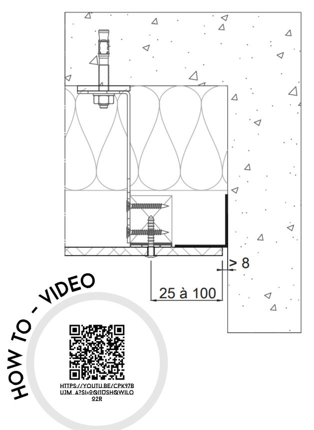
Always provide an expansion joint of at least 8mm when finishing an inner corner. Otherwise, changing weather conditions may cause the panels to expand against each other, resulting in possible breakage.
