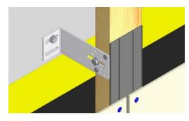
Support brackets should be made of galvanised steel.
