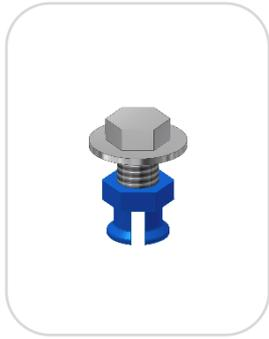
The panels are installed on a double metal substructure (minimal thickness profiles is 2mm, thickness panel hanger is 3mm) by means of a tension free undercut anchor, socket cap screw and washer.
