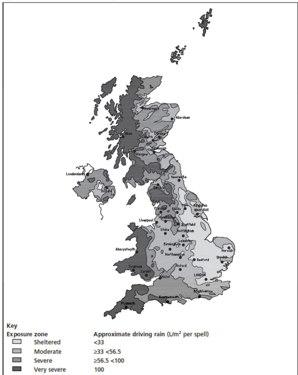
Figure 2 UK map of categories of exposure to driving rain
